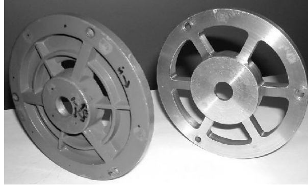
Figure 5.10: The original (left) and the new (right) cover shield.
